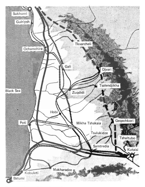
Figure 1. Scheme of the alternative routes for the Kutaisi-Sukhumi gas pipeline. Full line, maritime route; dotted line, median route; broken line, piedmont route.
